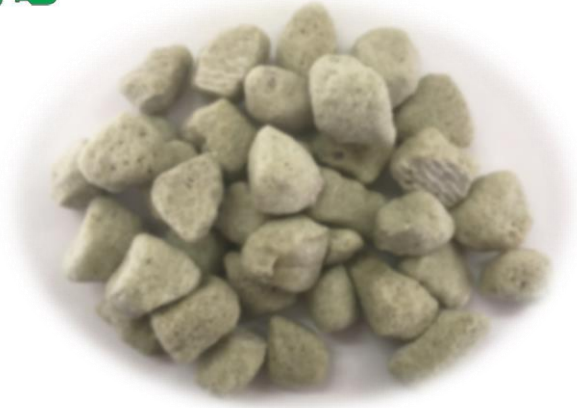
Manufacturing foamed glass, named "Porous Alpha"
